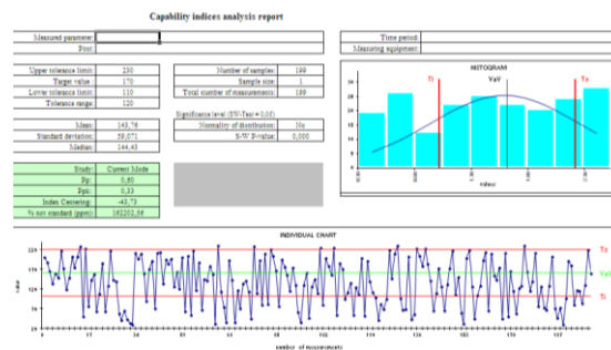
Figure 9: Control card before identifying and eliminating specific causes of variability.
